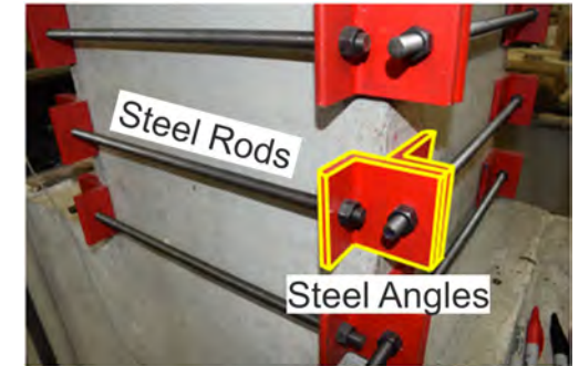
Proposed P.T. Clamps for retrofit and repair
