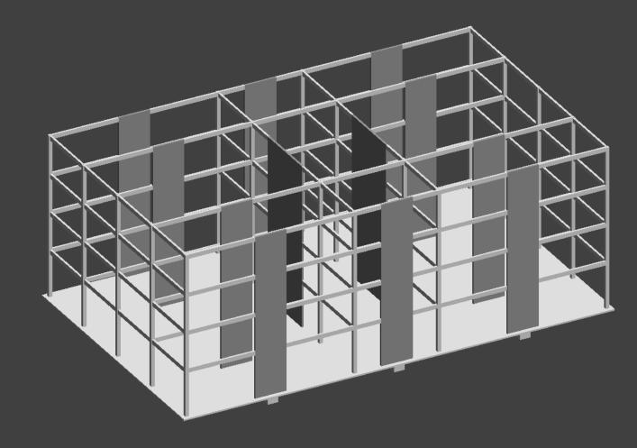
Build and validate the numerical models of these base-isolated buildings in OpenSees with lumped plasticity approach.
